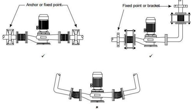
Stainless steel flanged pump connectors will exert a pressure thrust in service and must be anchored to protect adjacent pipework and equipment. Stainless steel flanged pump connectors will extend under pressure and must be anchored to prevent this happening.
