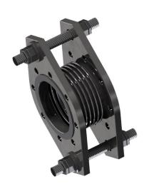
We can offer our Pump Bellows range both Tied and Untied. The tie bars will prevent elongation due to the internal pressure thrust. They are suitable for use on LTHW, MTHW, HTHW, Drinking Water, Steam & other gasses.
